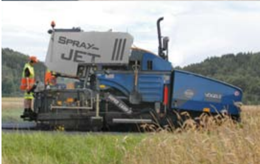
The SUPER 1800-2 with SprayJet Module handles all your resurfacing contracts in a highly efficient, economical and clean manner.
